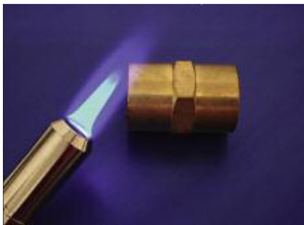
Figure 3. Photograph of broken brass valve that fractured due to the rapid application of heat. Note: a simple piece of brass is shown so as to not reveal the valve manufacturer.
