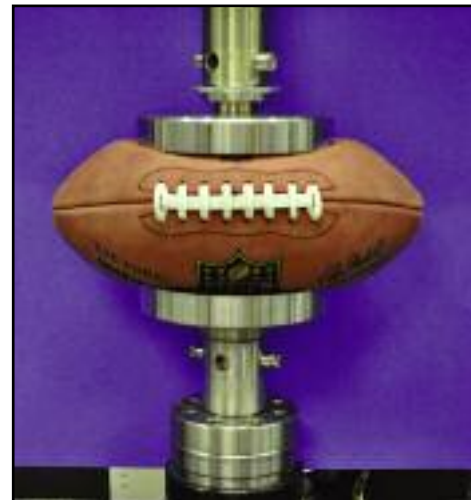
Figure 1. Photograph of a football being compressed to a 650-pound load in a test that was designed to simulate the effect of an aspect of game use.
