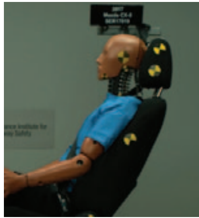
Figure 4: IIHS 10g acceleration rear-impact testing with an exemplar 2017 Mazda CX-5 showing pre-impact ATD position (left) and peak ATD rearward excursion (right).
