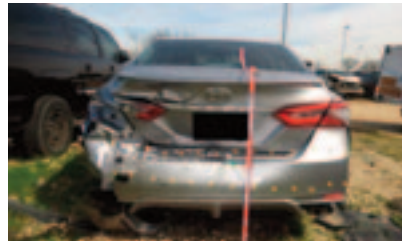
Figure 3: Crash Investigation Sampling System (CISS) database photo of a 2018 Toyota Camry following a 9.5-mph delta-V rear collision, recorded by Event Data Recorder (EDR).
