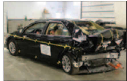
Figure 1: NHTSA 35-mph rear crash test of a 2015 Toyota Camry.
