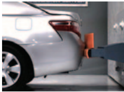
Figure 2: Insurance Institute for Highway Safety (IIHS) 6.5-mph rear crash test of a 2007 Toyota Camry.
