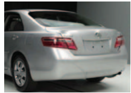
Figure 2: Insurance Institute for Highway Safety (IIHS) 6.5-mph rear crash test of a 2007 Toyota Camry.
