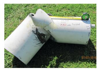
Figure 5. The upper failure showing buckling of the foremast towards the port side.
