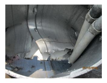
Figure 6. The vertical and horizontal fractures of the foremast viewed from the inside. Note the large, through-thickness weld nuggets along the right side of the seam weld.
