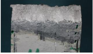
Figure 4. Macrophotograph of the lower fracture of the foremast, showing shear overload. There was no obvious indication of material defect or aggressive corrosion effects.
