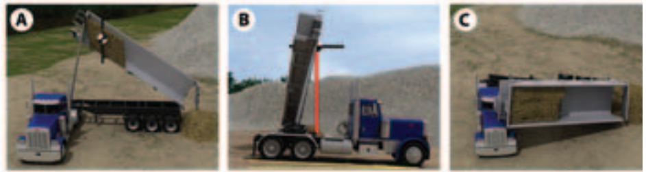
Figure 3: Articulated dump truck accident. Panel A shows the position of the tractor and trailer when the accident load is dumped. Note that the tractor is oriented nearly 90° to the trailer. The truck was parked on a slide grade, which tilted the trailer vertically as shown in panel B. Panel C shows the final position of the trailer after tipping over.
