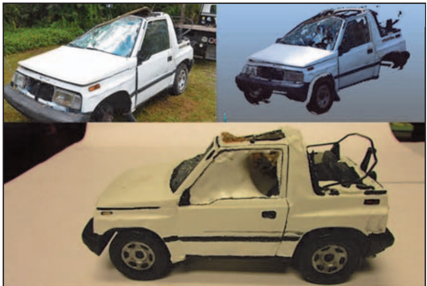
Figure 4: Upper Left = Subject Vehicle Upper Right = Vehicle Scan / Lower Right = 3D Printer Model
